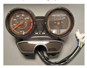
DRL indicator has been added on the new analog speedometer.
